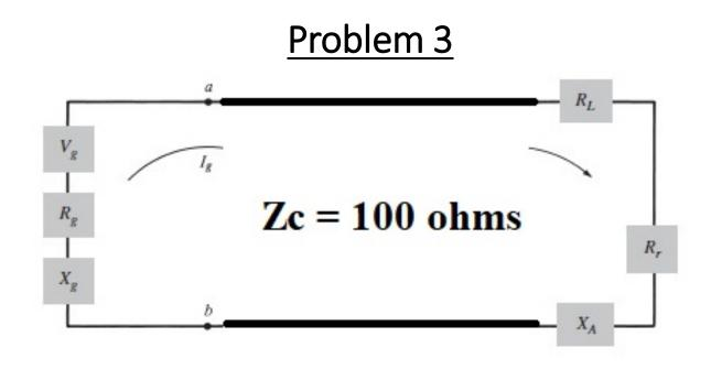
An antenna with a radiation resistance of 48 ohms, a loss resistance of 2 ohms, and a reactance of 50 ohms is connected to a generator with open-circuit of 10 V and internal impedance of 50 ohms via a  $\lambda/4$  – long transmission line with characteristic impedance of 100 ohms. Determine the power radiated by the antenna. Solution
